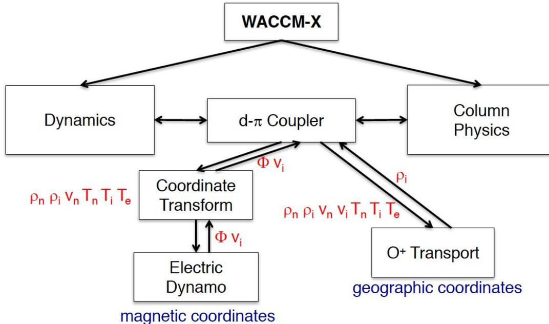
d- $\pi$  Coupler: dynamics-physics-ionosphere-electrodynamics (D-PIE) coupler
