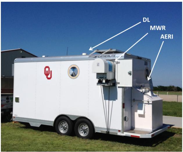
The CLAMPS1 facility is shown with the three main instruments annotated. Instrument specific information is included at the end of this document.
